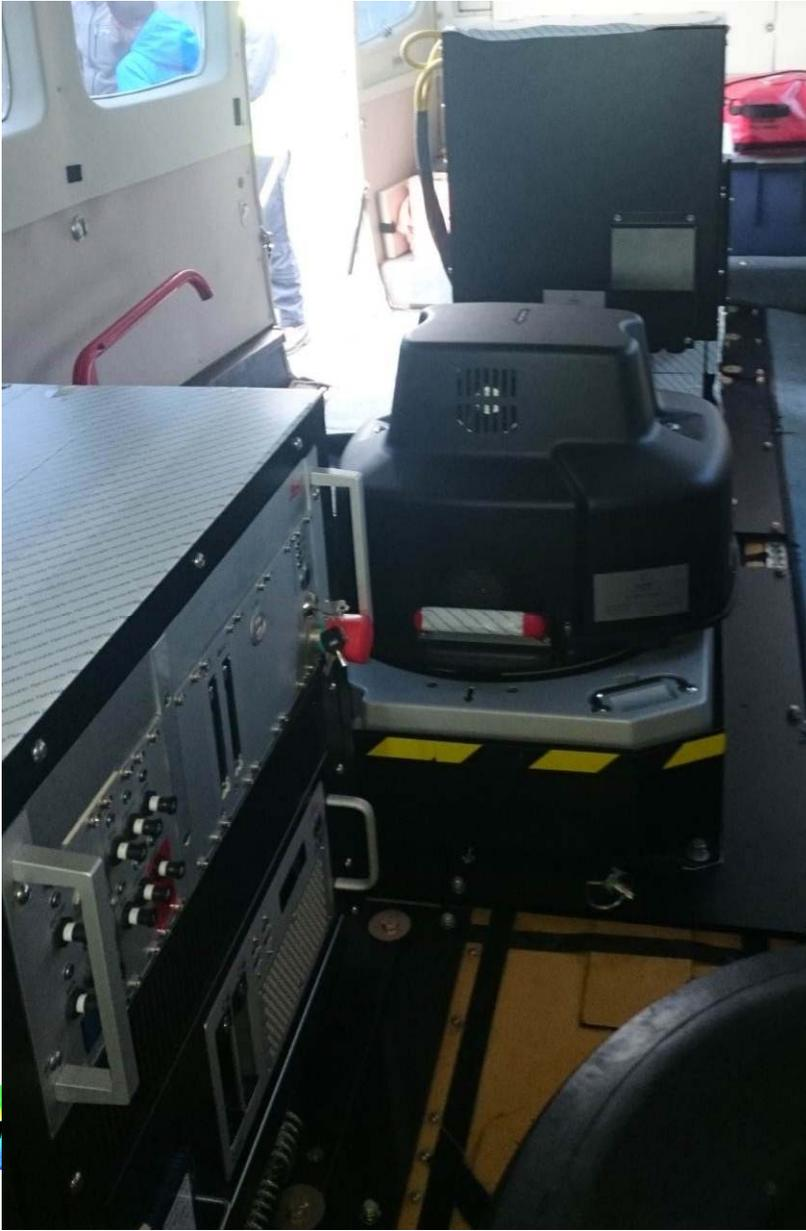
**HawkEye III = un lidar triple (topo, shallow, deep channels).**
